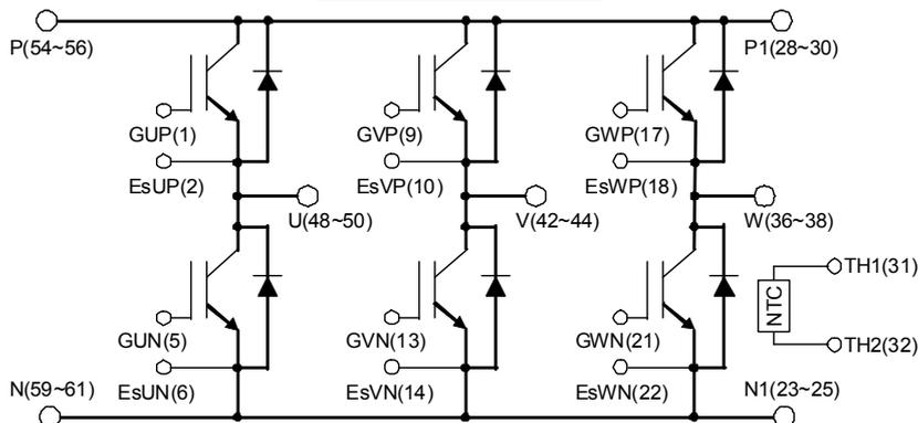
Caution: Each (three) pin terminal of P/N/P1/N1/U/V/W is connected in the module, but should use all each three pins for the external wiring.
