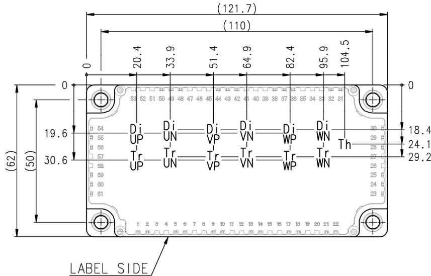
Tr\*P/Tr\*N: IGBT, Di\*P/Di\*N: FWDi (\*=U/V/W), Th: NTC thermistor
